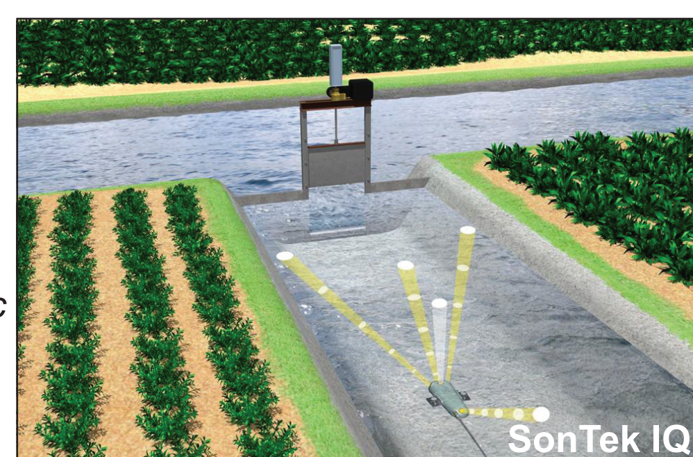
Figure 3. Illustrations of the two most typical configurations of the Acoustic Doppler meters to measure velocity in open channels (lateral, left); (bottom mount, right).
